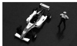
Figure 1. Single-seater racing car training for future professional drivers. Chassis: carbon monocoque as per FIA F3 2008 prescriptions; Engine: Renault K4MRS 1,600 cc; power: 140 bhp at 6,750 rpm; gearbox: SADEV 5-speed dog engagement with shift-cut gearbox; and weight: 470 kg.
